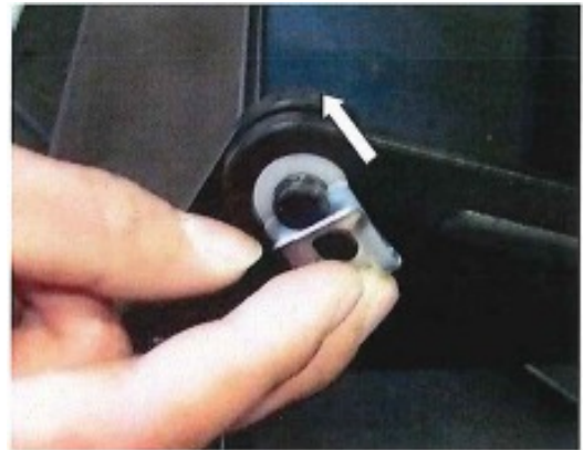
Secure assembly with safety clip
