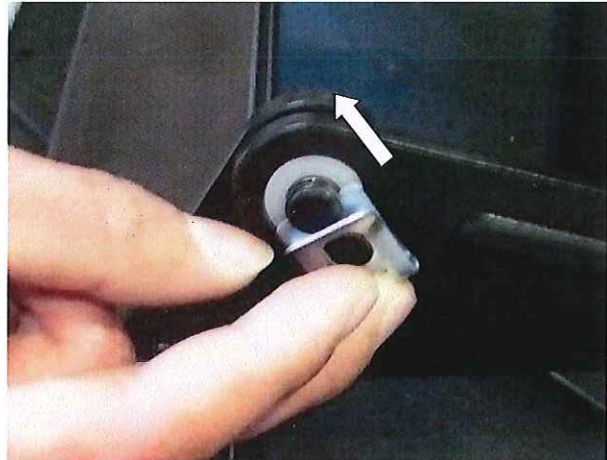
Secure assembly with safety clip
